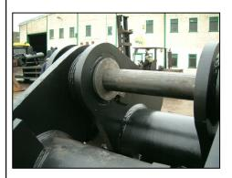
The Pulverisor hinges on the main dipper pin and comes complete with a longer hardened main pin.
