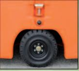
Superelastic tyres are fitted as standard, but cushion type are also available if required. Moreover, the NK-Series has the variable wheel base system that allows to increase the stability.
