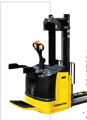
The MWP14/20F-1R stacker truck features 4-point contact chassis design with fixed lateral traction unit, a single castor wheel and tandem (2t) or single load wheels (1.4t). The side castor wheel is adjustable in height to compensate for possible wear on the traction wheel. This creates maximum load stability and excellent residual capacity, both of which are primary requirements
