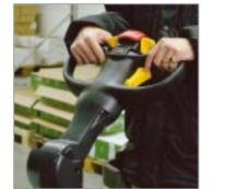
• The ergonomic central positioned tiller has an exclusive electric power steering system. It allows constant fatigue-free manoeuvring of the tiller within 2 x 75° with traction wheel moving 2 x 90°. It is particularly efficient in picking up pallets that are placed against walls or lorry
