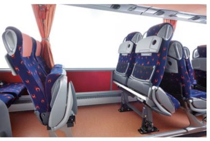
With the cinema/sliding seat combination, folding up the cinema chair seat cushion and folding forward the sliding seat creates space on the platform for a stroller or pram.
