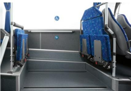
On request, **four individual folding seats** can be integrated as well. When they are folded up, there is more than enough space for a stroller or wheelchair. The folding seats are fitted with lap safety belts.
