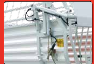
Optionally with hydraulic door opener , for convenient opening of the door from the driver's seat.
