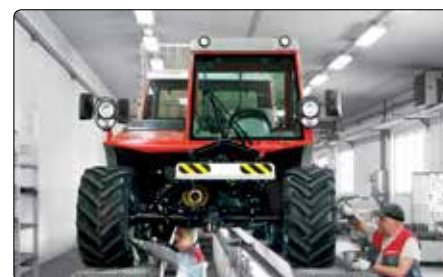
In the end-of-line check and the finishing department, all machines are thoroughly checked once more and prepared for shipment to their future owners.
