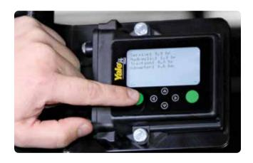
In addition to limiting truck access to trained and authorized operators, Yale Vision can track training updates, provide impact monitoring and alerts, and incident data for route optimization. It also requires the completion of OSHA pre-shift checklists before the truck will operate.
