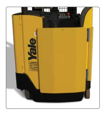
You should assess your workplace environment and evaluate whether potential intrusion hazards warrant the selection of a rear guard door for your stand-up lift trucks, compared with the risks posed by a delay in exiting a unit equipped with a rear guard in the event of a tip over or off-dock accident.
