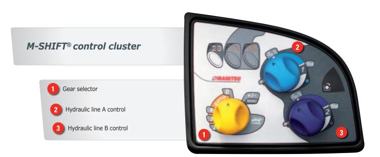
When making heaps of silage or picking up cereals, you may decide to go no higher than third gear. In this case, you select 3 and your MLT 840 will take care of the gear changes, quickly and smoothly, but will never engage a gear higher than third.
