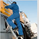
The integrated ladder provides the driver with safe access to the slewing platform and the lift cab.
