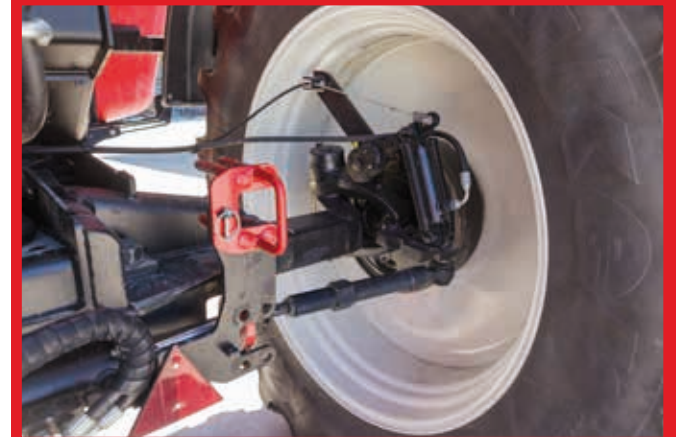
Pivot steering for 54° steering angle and exact track following..
