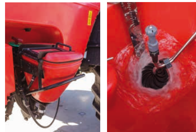
High performance filling, liquids and powders are easily dissolved and mixed with the PowerPowderJet.
