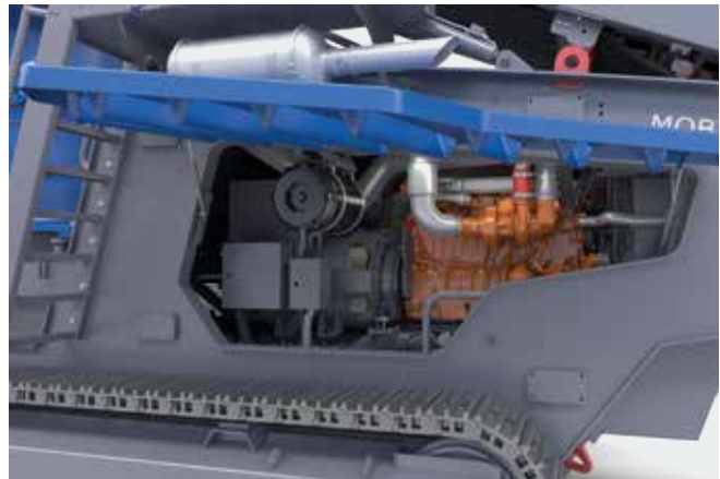
> MCO 11 PRO - convenient access to the engine compartment, refuelling possible from the ground
