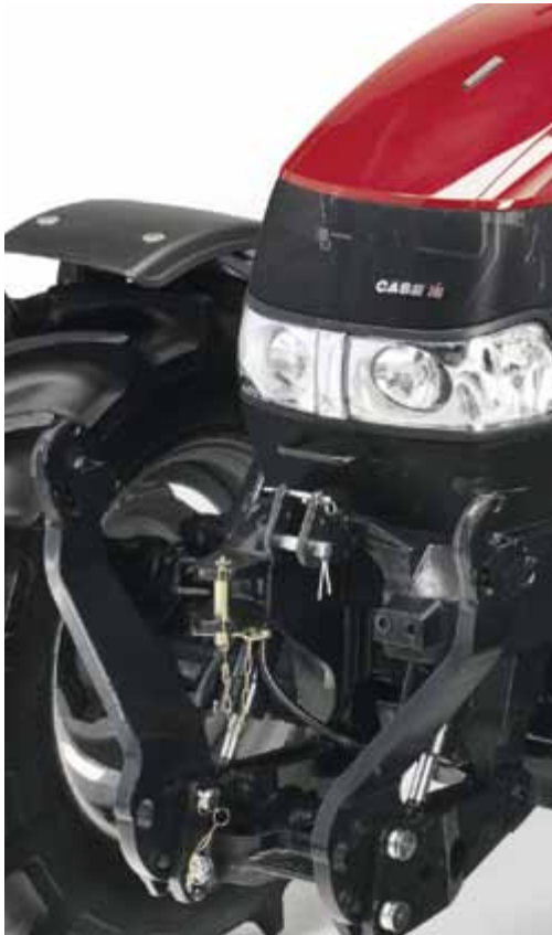
Seamlessly integrated front linkage with a lifting power of up to 3,800kg. Optional available front hitch management for Maxxum Multicontroller and CVX.
