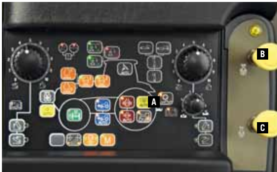
... the Maxxum Multicontroller and Maxxum CVX. A – Automatic PTO controls B – Front PTO on/off C – Rear PTO on/off
