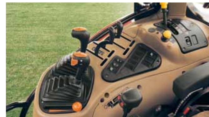
Pure functionality for Maxxum tractors. You can choose between a 2-speed Powershift transmission with 24x24 speeds and the ...
