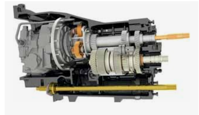
CVX transmission - stepless drive between 0-50kph.
