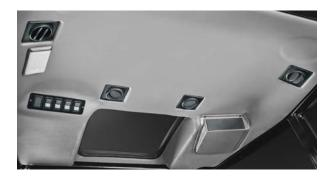
The roof panel is pre-wired for a radio and air-conditioning, and features a roof hatch.
