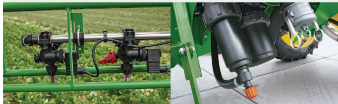
Choose between two types of edge nozzle holder.
