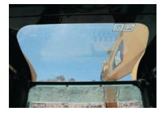
Viewing Area. To maximize visibility, all glass is affixed directly to the cab, eliminating the use of window frames. Choice of fixed or easy-to-open split front windshield meets operator preference and application conditions.
