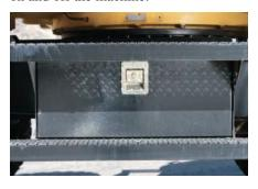
**Storage Box.** There are two toolboxes integrated in the steps of the undercarriage. Additionally, there is a waterproof storage box integrated into the upper structure steps.
