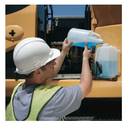
Ground Level Maintenance. Caterpillar designed its D-Series Wheel Excavators with the operator and service technician in mind. Gull-wing doors, with pneumatically-assisted lift cylinders, effortlessly lift up to allow critical maintenance to be performed quickly and efficiently while maintaining operator safety.
