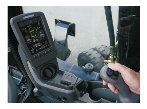
**Control Settings.** There are 2 selectable control settings and one automatic travel setting. The new automatic travel mode is activated with a button in the right hand console. In this setting, the transmission will automatically shift up or down, depending on the speed conditions. The operator can choose the best power setting for both engine and hydraulic power versus fuel efficiency.
