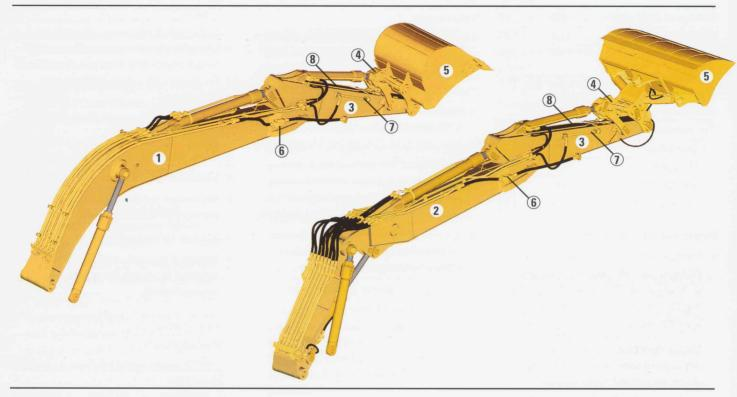
Booms and sticks are built with large cross sections for maximum strength and durability while keeping the weight as low as possible to enhance payloads and lifting capacity.
