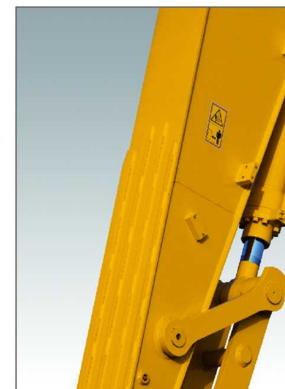
Arm rib reinforcement
