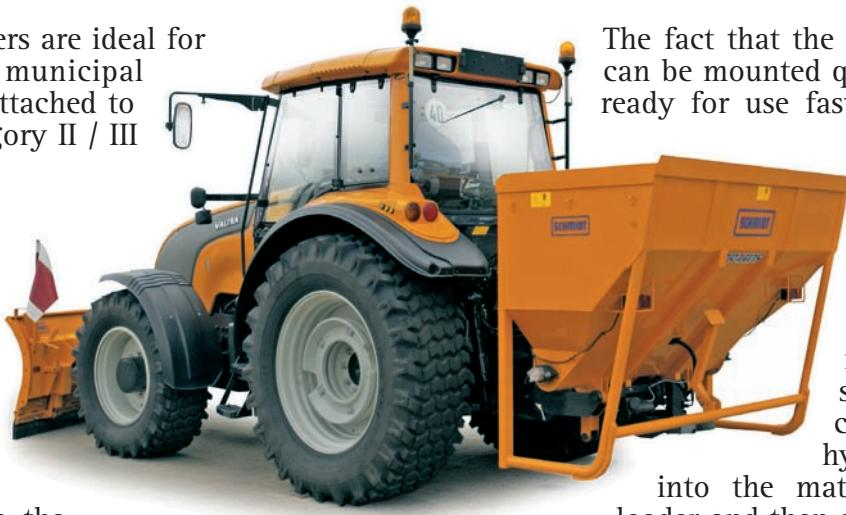
The fact that the TRAXOS spreaders can be mounted quickly makes them ready for use fast. The self-loading facilities allow drivers to single-handedly load the spreading materials onto the spreader enabling them to start work immediately. The spreading material container is tipped hydraulically, pushed into the material like a front loader and then swings back.
