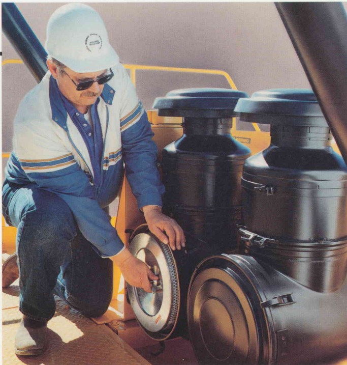
Air cleaner restriction sight gauge / service platform.
