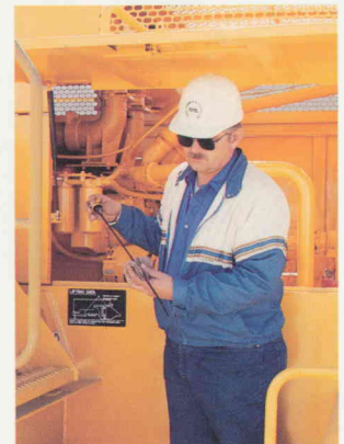
Quick-connect, remote pressure check ports save time and labor.
