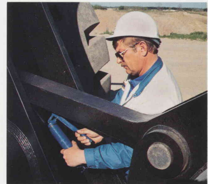
Grease fittings grouped so they can be lubed from four ground level locations.
