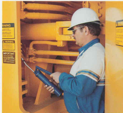
Center hinge lube manifold.
