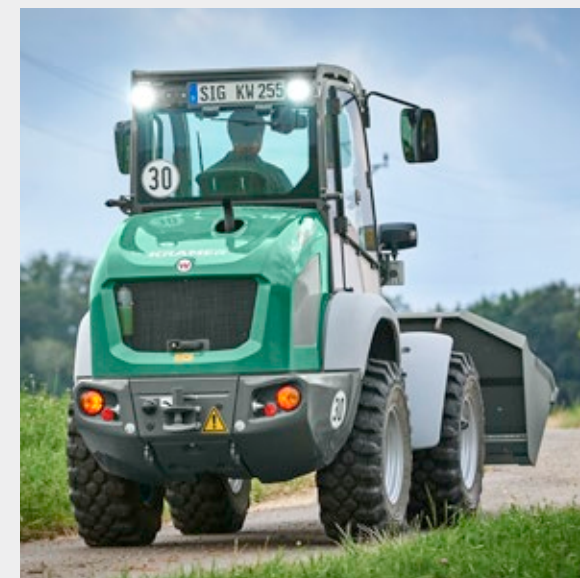
Front wheel steering for increased stability during transport trips.
