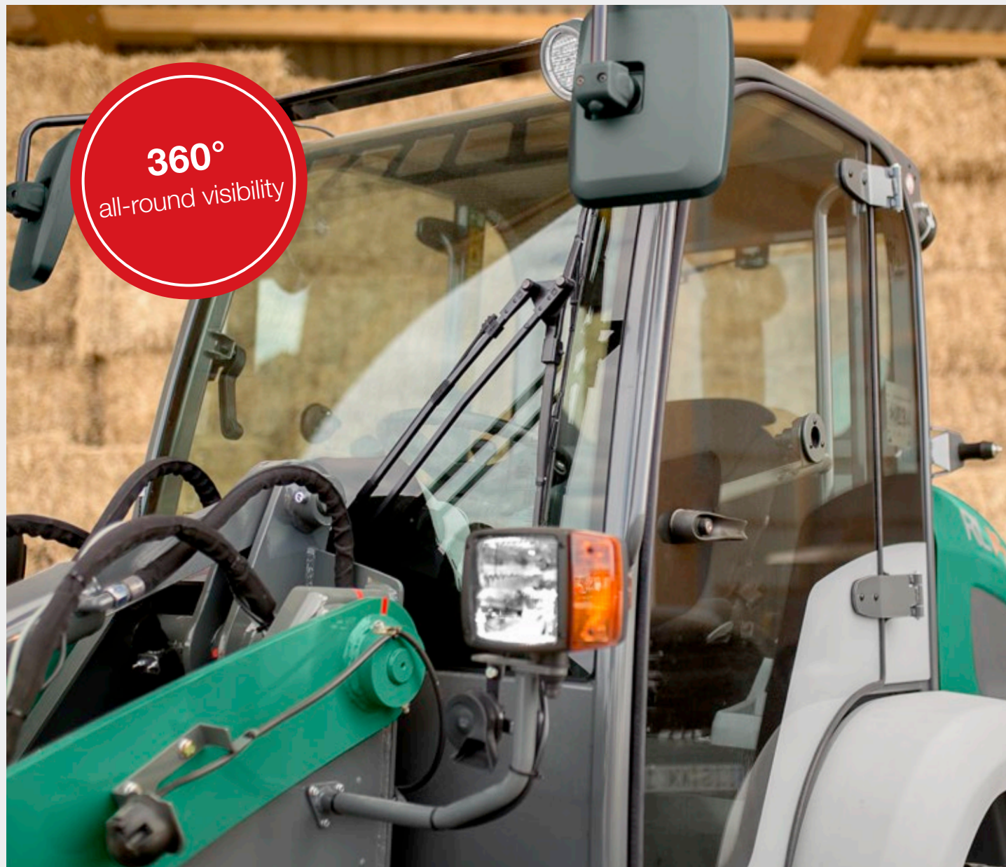
Panoramic cabin for an excellent overview of the attachment and the working environment.
