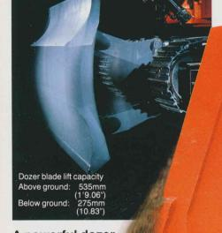
A powerful dozer blade for earthmoving and levelling
