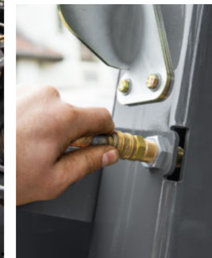
Three integrated compressed air connections permit important parts of the vehicle to be dry cleaned directly in the field.
