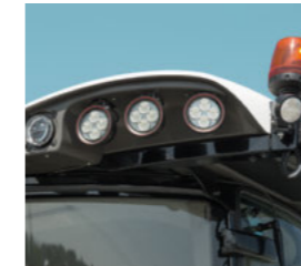
3 pairs of work lights in the roof, driving lights in the front of the roof, side finder lights and a rotating beacon.
