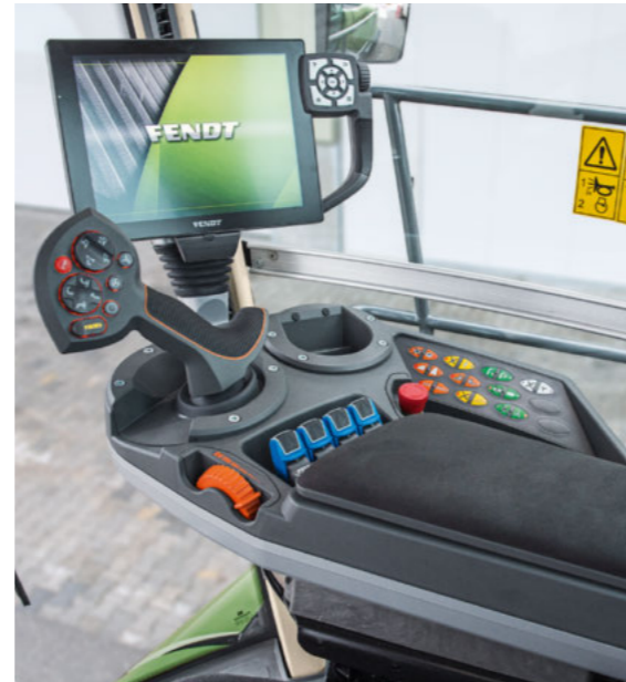
The practical right armrest, which is very popular with Fendt tractor drivers, has been adopted and adapted to the forage harvester.
