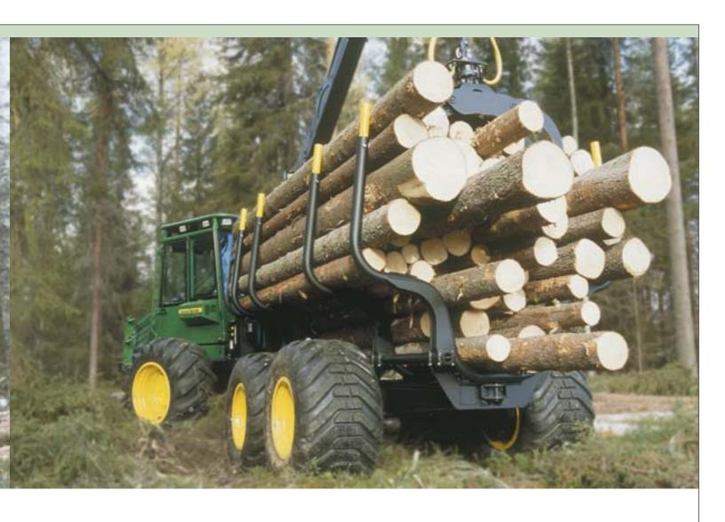
The John Deere 1010 forwarder efficiently improves the environmental friendliness of harvesting work. Its low centre of gravity, smooth transmission and wide tyres minimise ground pressure and the effects of the terrain. The efficient John Deere engines have low emission and conform to the latest emission regulations.
