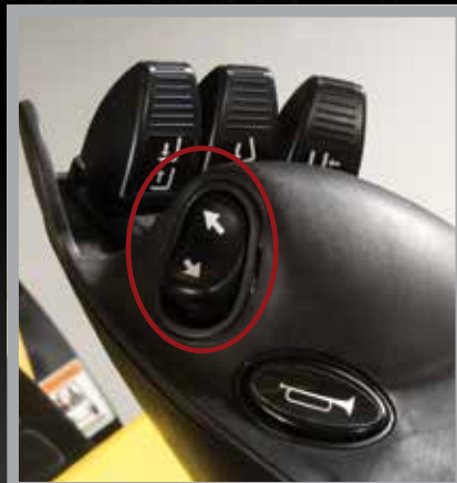
Electro-hydraulic controls with TouchPoint mini-levers
