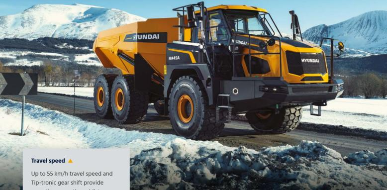
Tip-tronic gear shift provide smoother operation whilst maintaining maximum momentum.
