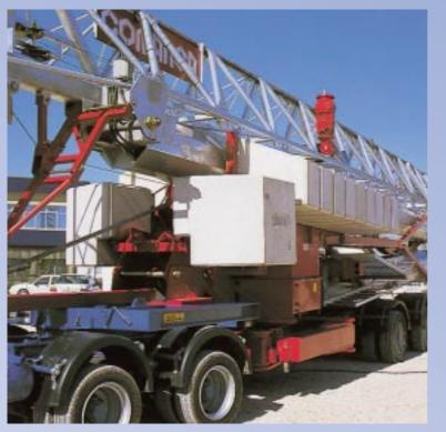
Thanks to the folding counterweight system, the weight is evenly transmitted to the axles to permit transport of the crane FULLY BALLASTED.
