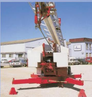
No external equipment necessary; the HT-30 is quickly and safely levelled using the central hydraulic system of the crane.
