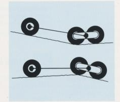
power to the rear wheels. The limited slip differential and differential locks reduce slippage to a minimum, for better traction and longer tire life. This improves gradeability, so the equipment can handle steeper slopes to shorten hauling distances and cycle time, particularly in quarries. And the turning ring articulation system increases maneuverability in confined areas, for greater productivity.
