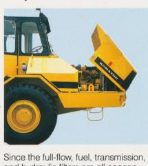
and hydraulic filters are all concentrated on the left side of the machine, replacing any of them is quick and easy. The fuel and hydraulic tanks are positioned low for easy refilling. The engine bonnet of the HA270 tilts for greater service
