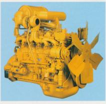
A dependable combination of the newest KOMATSU diesel engine and a ZF transmission power the permanent six-wheel drive. Komatsu's S6D125 diesel engine delivers a maximum of 248 HP at 2200 RPM and features a direct-injection system to maximize fuel efficiency. And the full powershift transmission with automatic converter lock-up provides easy gear selection.
