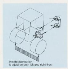
The articulated frame hydraulic steering of the HA250 delivers instant response for precise positioning. It can swing a full 45° to the left or right. This enables the HA250 to operate smoothly in narrow places and tight corners such as underground mines and steelworks.
