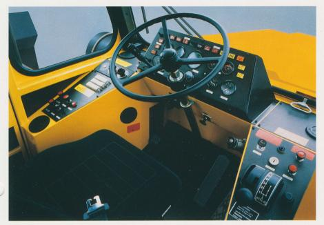
The cab is built to current ROPS standards, with full soundsuppressing, heat/vibration insulation and an adjustable suspension seat. The driver sits directly above the middle of the front axle, where movement due to uneven terrain is minimized. The cab has two side doors providing excellent access and assures
