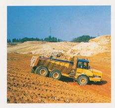
With unique features like its permanent six-wheel drive and turning ring articulation system, the HA250 guarantees outstanding performance, economy and reliability, whatever the terrain. The permanent six-wheel drive keeps the power in contact with the ground at all times to keep the truck moving even in the toughest situations. It uses a single driveshaft to a pivoting rear tandem and differential to transmit
