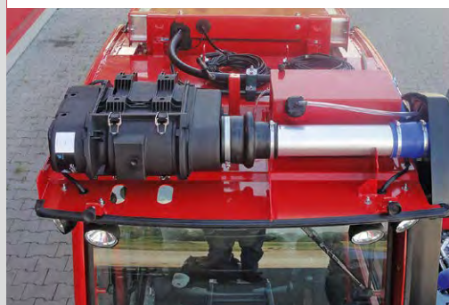
The complete intake area and the air filter unit are located above the driver's cab.
