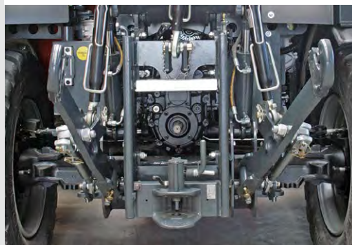
Solid rear lifter with hitch block that is adjustable for height
