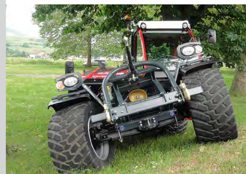
The high-placed articulated joint gives the vehicle high stability to prevent tipping over. The arrangement of the articulated joint gives the front axle an extremely large swinging range
