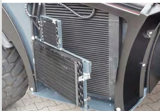
Cooler packaged arranged on the side allows easy cleaning by swivelling out the individual cooler segments without the need for tools.
