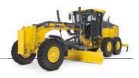
Hydraulics622G/GPTypeClosed-center, pressure-compensated load-sensing (PCLS), variable-displacement piston pumpMaximum Pump Flow212 L/min. (56 gpm)Maximum System Pressure18 961 kPa (2,750 psi)
