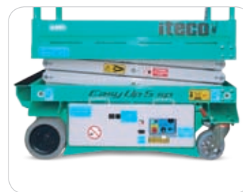
Pothole protection steel shoes welded nearby the wheels.
