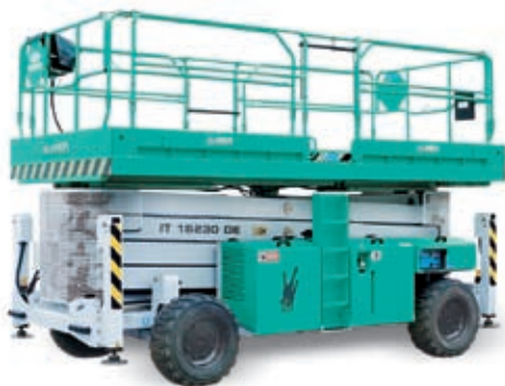
Automatic hydraulic levelling outriggers
