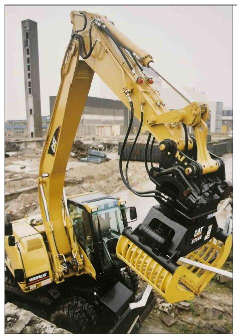
Caterpillar G310B, G315B and G320B Multi-Grapples are equally well suited for demolition of brick and wood structures. These Multi-Grapples are extremely effective for sorting and loading a variety of different materials as found in demolition and scrap piles. The speed, dexterity, clamping force and rugged construction make these Multi-Grapples ideal tools for
