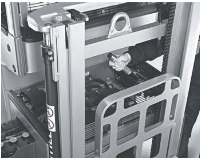
Battery change over the side as standard for highest availability and ergonomics
