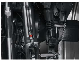
**SPRING-MOUNTED CAB**All Forterra models have the cab springmounting system to maximize operator's comfort.
