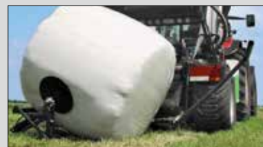
Bale turner, unloading the bale on its flat end
