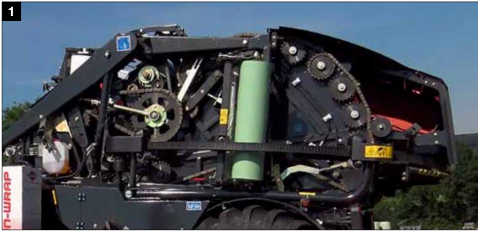
Robust driveline with high quality IWIS chains
