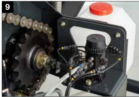
9 Beka Max continuous chain oiling system
