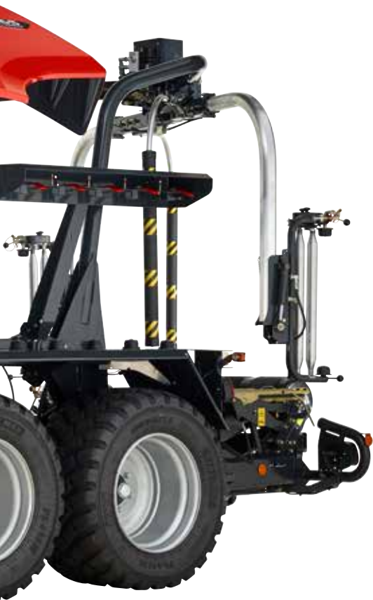
9 Beka Max continuous chain oiling system
