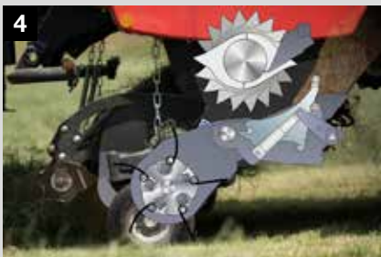
4 During the process, the rotor speed is monitored constantly. The rotor movement indicates when the intake system is cleared again, and triggers the next step in the process
