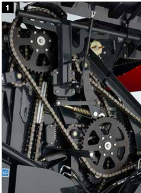
Robust driveline with high quality IWIS chains
