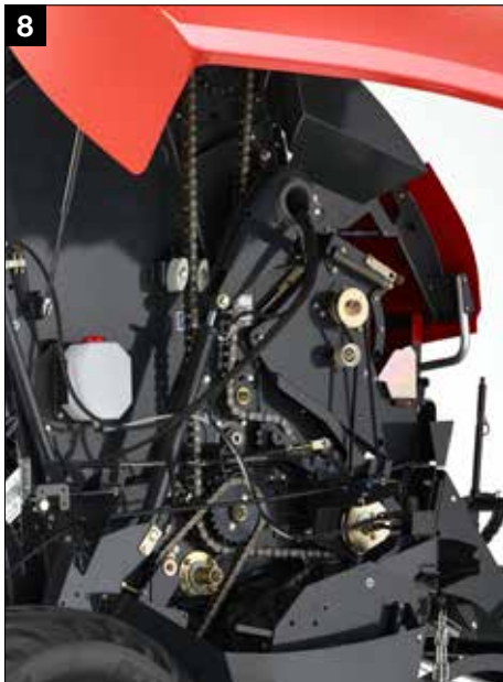
8 Robust driveline with high quality IWIS chains + 1¼" 20BH primary driveline with chrome hardened pins
