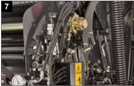
7 Proportional valve for in-cab density control
