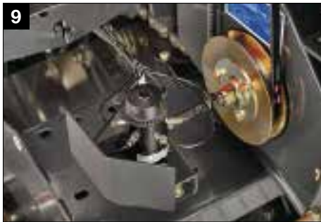
9 Beka Max continuous chain oiling system
