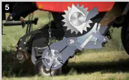
5 When the correct rotor speed is measured, first the dropfloor system is brought back into position. Thanks to the automatic process, this time is brought back to a minimum
