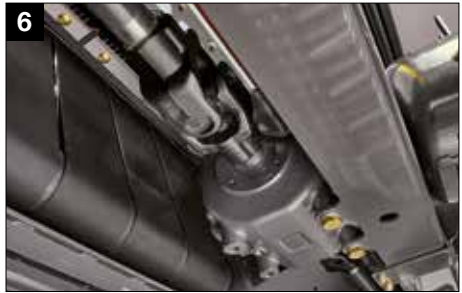
6 Heavy duty cross joints in the drive axles
