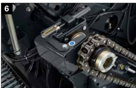
6 Standard hydraulic rotor disengagement
