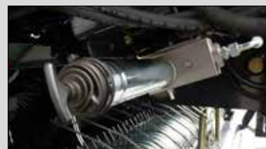
Beka Max automatic bearing greasing system
