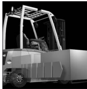
Lateral battery exchange
