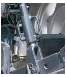
▲ Rugged 3-point hitch provides impressive lift, while a turnbuckle leveling system, telescoping stabilizers and fixed link ends at the lower arms allow for easy attachment.
