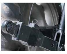
▲ Standard mechanical lower-link draftsensing system on FARMALL tractors provides position and draft control.
