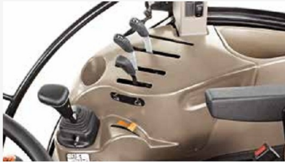
Up to three mechanical rear remote valves are available for the Farmall A range.
