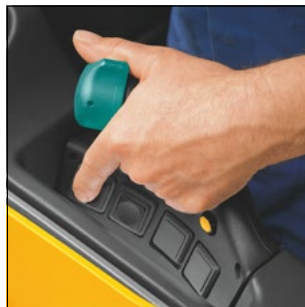
ESD 120: Control panel for speed regulation and lift function
