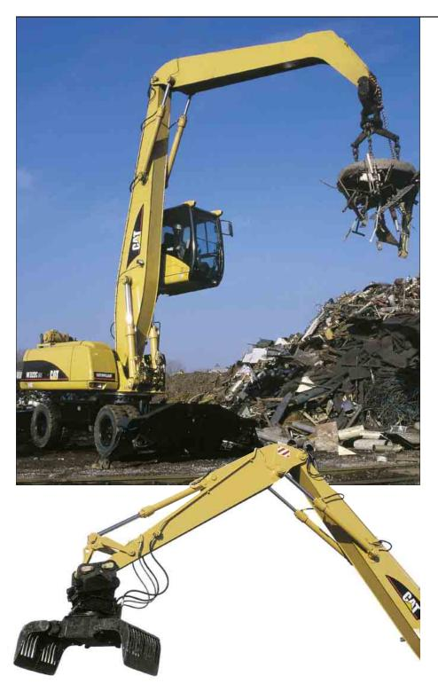
MH Booms and Sticks. The M318C MH boom (6200 mm) and M322C MH boom (6800 mm) have been redesigned to handle increased lifting capacities. The new stick range offers leading side plates to maximize protection of hydraulic lines. The lines are fitted in between the two side plates offering protection from damage.
