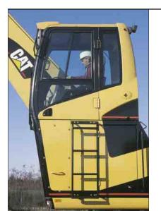
Fixed Cab Riser. The fixed cab riser offers a very stable and comfortable method to raise the cab. The fixed cab riser lifts the cab by 1200 mm to offer better viewing to all sides. Well-positioned steps lead continuously from ground level to the raised cab. In shipping position, the cab is unmounted to meet national road regulations.
