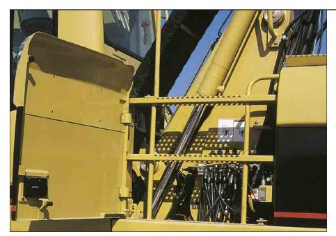
Extended Service Intervals. M318C MH and M322C MH service and maintenance intervals have been extended to reduce machine service time, increase machine availability and reduce operating costs. Using S•O•S hydraulic oil change intervals can be extended from 2000 hours to 4000 hours. Engine coolant change intervals are up to 6000 hours when Cat Extended Life Coolant/Anti-Freeze is used.
