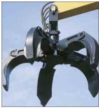
**Orange Peel Grapple.** The most common tool for material handling applications, this grapple is available in a range of sizes and provides a solution for a wide range of material types. The grapple is free swinging and has unlimited left and right rotation.
