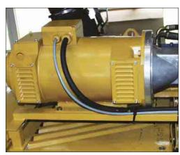
**Generator Set.** The hydraulically driven generator set (12.5 kW) offers electric power needed for magnet applications. With a priority flow valve, the power from the generator is provided at a constant level.
