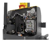
Sealed AC motor, controllers and connectors
