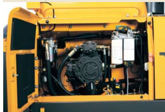
• Easy access for hydraulic pump filters.
