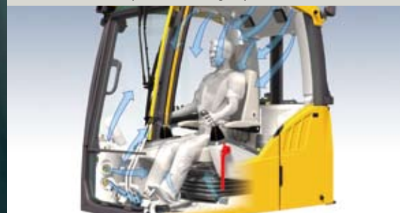
• Industry's highest heating/cooling capacity with 14 vents.
