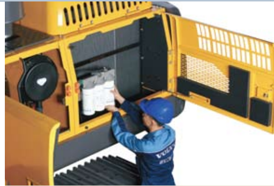
• Simplified, ground level service access.
