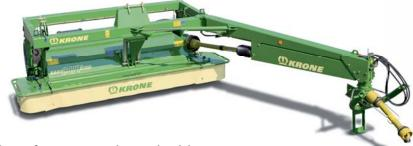
the world. Compact by design, these machines feature a robust double frame and a side-mounted drawbar for mowing round and round.
