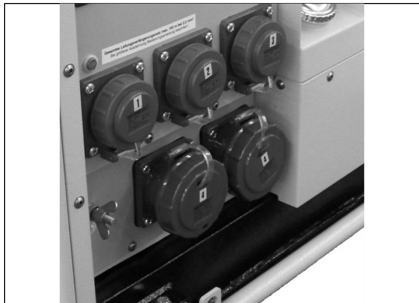
Fig. 4-3: Connecting up to consumers
