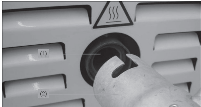
Figure 5-11: Connecting up the exhaust hose
