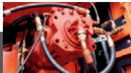
Hydraulic pump The main pump has a capacity of 2 x 436 l/min
