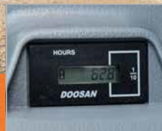
Hour meter (from ground level)
