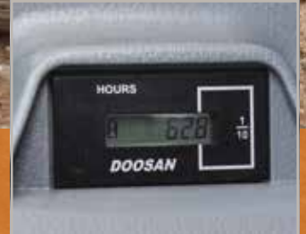
Hour meter (from ground level)
