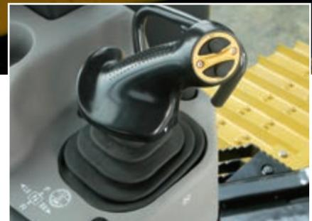
PCCS-Bedienhebel (Palm Command Control System)
