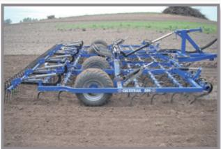
Heavy duty trailed seedbed cultivator Working width 5 and 6 m
