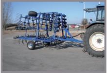
Despite its wide working width CultiTrail is only 2.5 m wide in Transport position. Folding and unfolding is controlled hydraulically from the tractor seat, which makes the job very easy for the operator.
