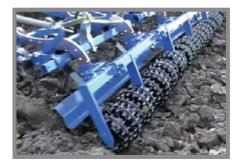
A 330/300 mm Crosskill roller can be fitted at the rear of the cultivator. The soil is consolidated and the working depth is controlled very precisely. Made out of steel, the weight is limited, maintaining the superb cultivation effect of the Crosskill ring style.
