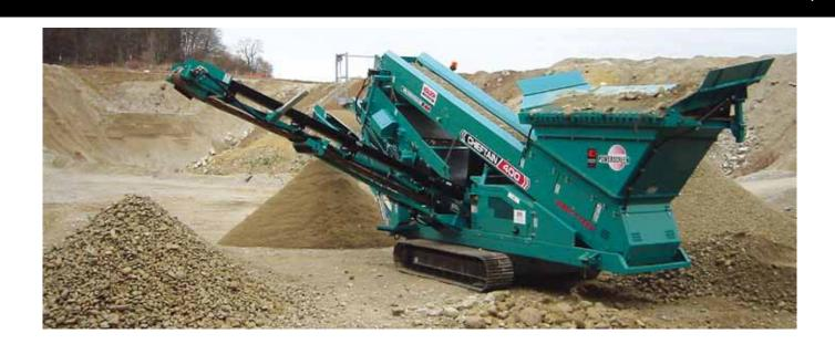
The Powerscreen® Chieftain 400 and 600 are designed for smaller end users or contractors looking for an affordable entry level screening unit. These entry level machines share many of the class leading features of the larger models in the range including remote tipping grid, main conveyor, high performance 2 deck screen and hydraulically folding conveyors.
