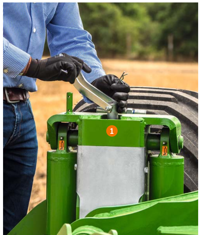
Working depth adjustment on the depth wheel
