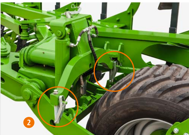
Adjustment of the plough tilt
